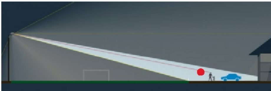
Intensity towards the observer: this concerns the luminous intensity emitted by the luminaire in the direction of the observer.
